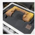
Sand Casting Process Francis Manufacturing Company produces quality castings using the green sand process. A pattern is used to create an impression using a mixture of sand, water and organic compounds. A sand mold is comprised of two parts;
